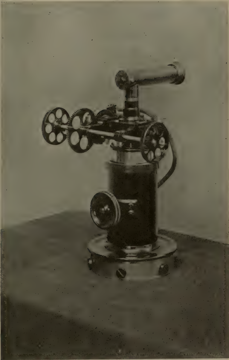
FIG. 39. The Transit Micrometer. (Coast and Geodetic Survey.)
